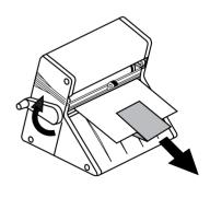
Install feed tray and trim off excess film using cut blade.
